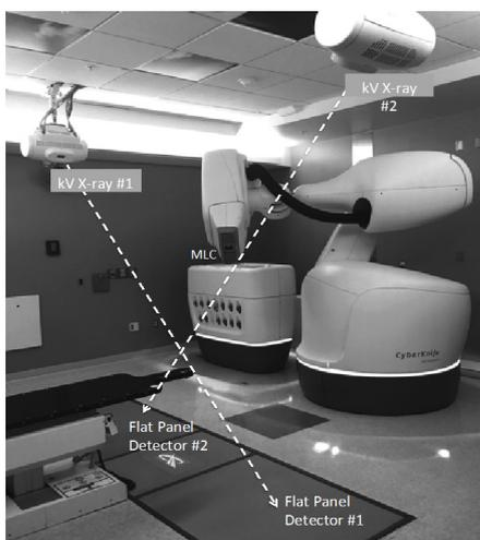
**Figure 3** Illustration of the latest robotic CyberKnife® M6™ system with the tertiary MLC system attached to the beam exit port. Rapid 2D stereoscopic imaging is accomplished by a pair of in-room X-ray imagers as shown.
